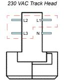
The 230 VAC three circuit head uses three Hots and one Neutral selectable
