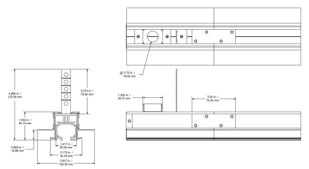
Figure 1: Spackle Flange for 2-Circuit Track (120V)
