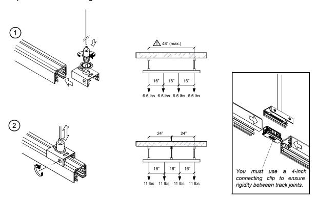
Figure 7: Pendant Clips for Track-to-Track Connections
