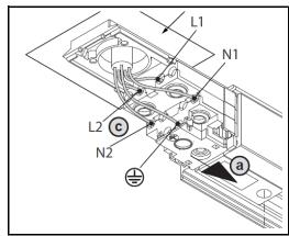
Figure 9: Wiring 120VAC System
