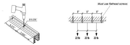
Figure 4: Drilling Mounting Holes
