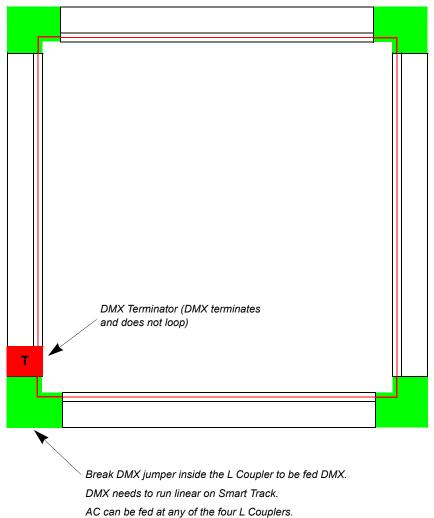
DMX can be fed at any of the L Couplers and the terminator placed at the opposite side.
