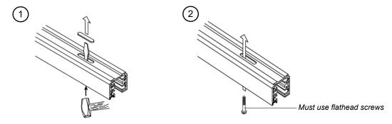
Figure 3: Pre-Punched Mounting Holes
